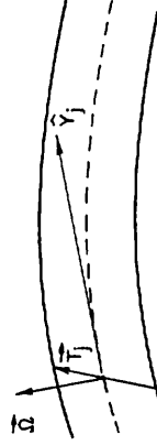
Figure 11.14 The vector thickness at a Loof node must have zero component along the edge, to avoid spurious rotations
